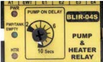
WATER LEVEL REGULATOR An electronic device receives input signals from sensor probes placed at critical water levels within the boiler shell.
